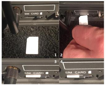
Figure 2-13 Installing SIM Card and Engaging the Lock
