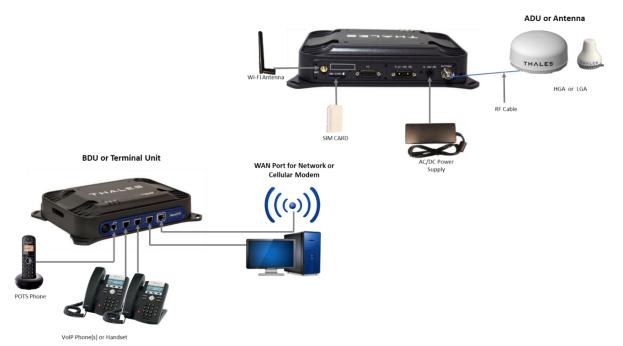
*Figure 1-1 Thales VesseLINK<sup>™</sup> System with Accessories*
