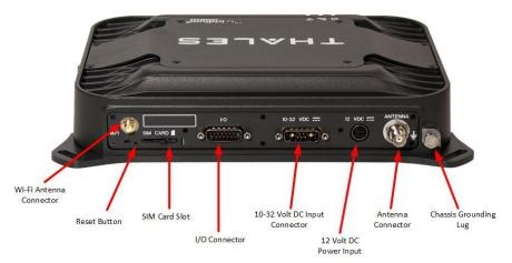
Figure 1-5 Below Deck Unit (BDU) Back Panel Detail
