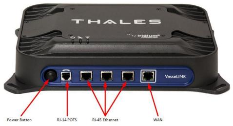
Figure 1-4 Below Deck Unit (BDU) Front Panel Detail
