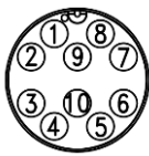
Figure 25: AUX connector pin out
