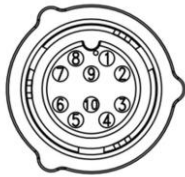
Figure 26: AUX cable pin out
