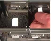
Installing SIM card and engaging the lock
